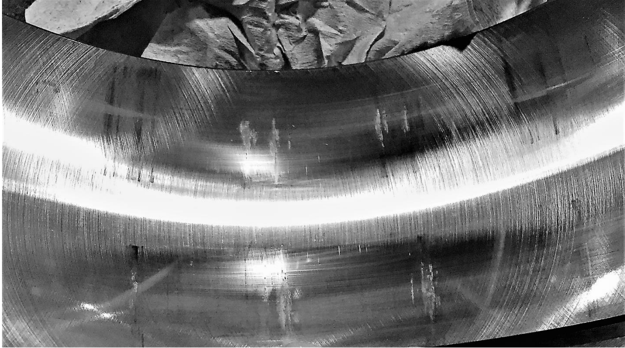
Figure 6. Outer race defect of a bearing on the tending side of a lower calendar roll.
